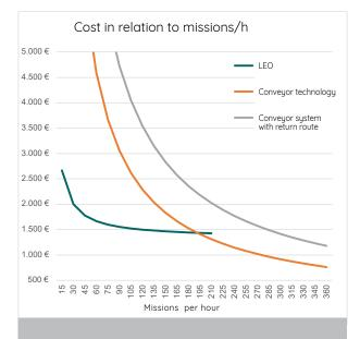
The graph shows the investment costs for the number of trips per hour. It compares LEO costs with a one-way conveyor route and a conveyor system with a return route. LEO costs are constantly at a low level and only undercut by conveyor technology at high throughput rates. LEO applications with more than 200 missions are technically not feasible.
