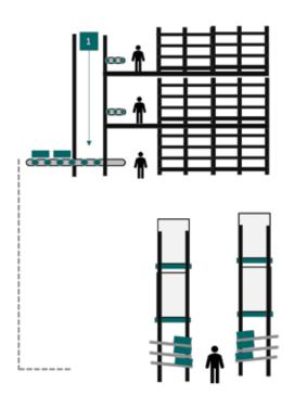
Order picking area featuring BITO carton live storage for fast order picking. A powered conveyor line mounted on the racking short side passes empty containers to a LEO flow vehicle. It is also possible to use the conveyor line to move finished orders to dispatch.
