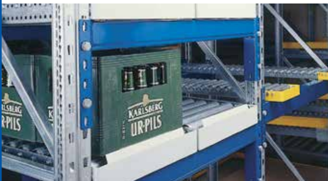
A rigid stop profile at the loading side stops backfeeding – profile with forward incline for easy loading
