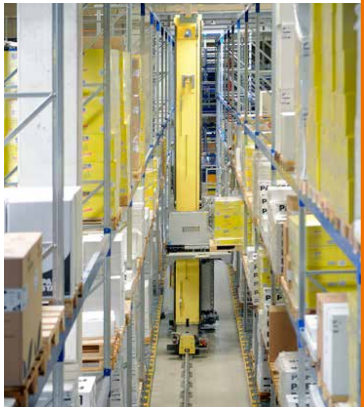
Papstar, static pallet storage on the upper levels, while pallets that are fed into the live storage floor level move down the lanes to the picking face.
