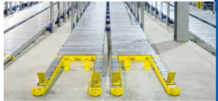
2-track segment for hand pallet truck retrieval
