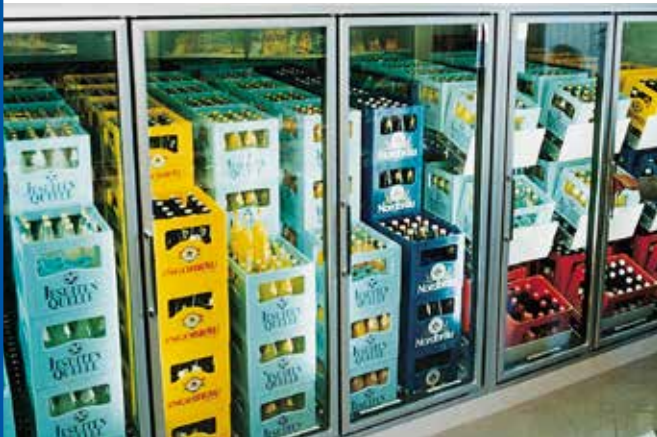
Lanes with front incline are ideal for single bottle picking, whereas straight lanes are preferred for beverage case picking
