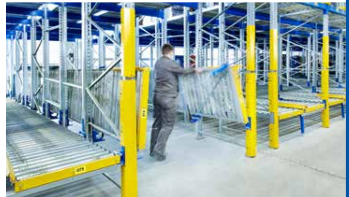
Tiltable/hinge-up roller conveyor segment
