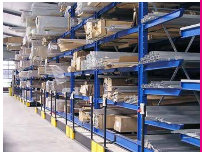
Mobile cantilever racking storing long loads
